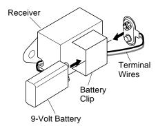
Figure 37 - Installing Battery in Receiver
